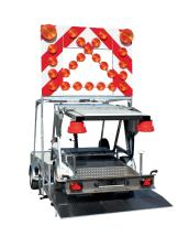
Brought quickly and efficiently to the scene with just one towing vehicle mobile warning trailer AM 4 TL carrying the mobile prewarner MV-LED.
